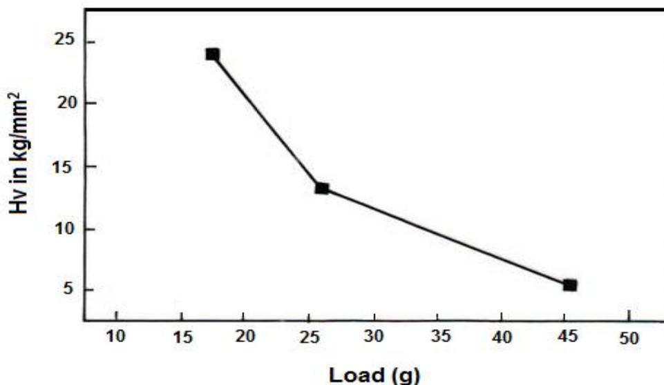
Figure 8. Variation of hardness with applied load of DNMDC - Cd
