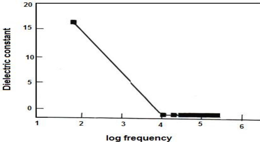
Figure 11. Variation of dielectric constant with log frequency
