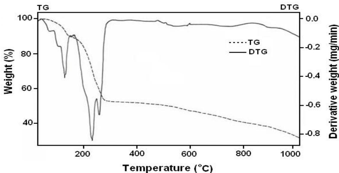
**Figure 3.** TG-DTG curve DNMD-Cd crystal
