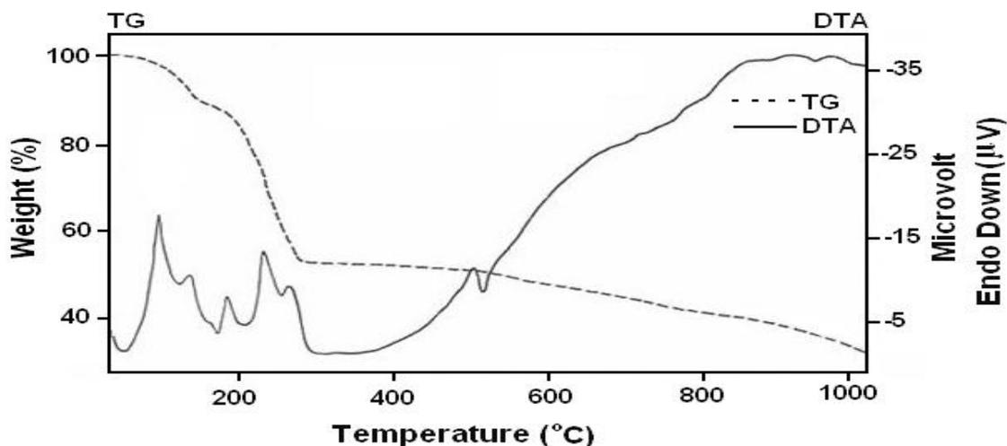
Figure 4. TG-DTA curve of DNMD-Cd crystal
