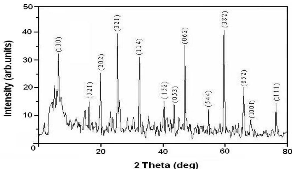
**Figure 2.** Powder X-ray diffraction pattern of DNMDC-Cd crystal
