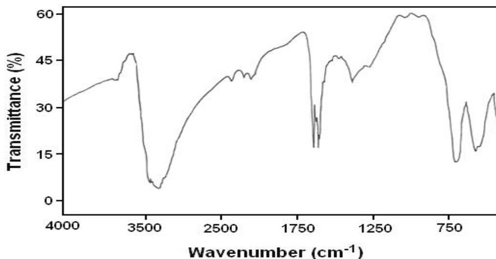
Figure 7. FTIR spectrum of DNMDc-Cd crystal
