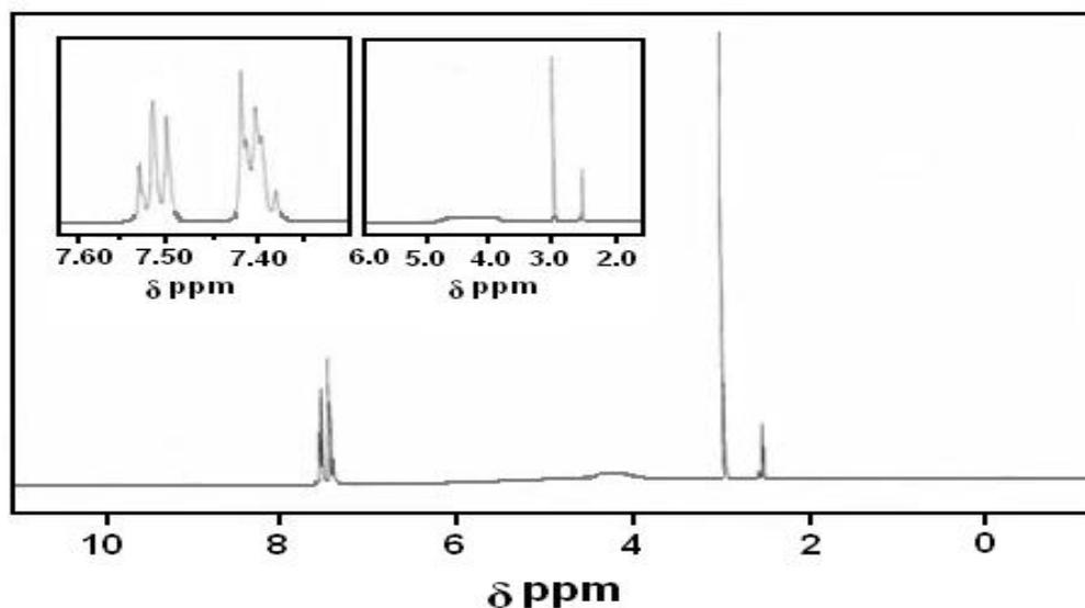
Figure 6.  $^1\text{H}$  NMR spectrum of DNMD-Cd crystal
