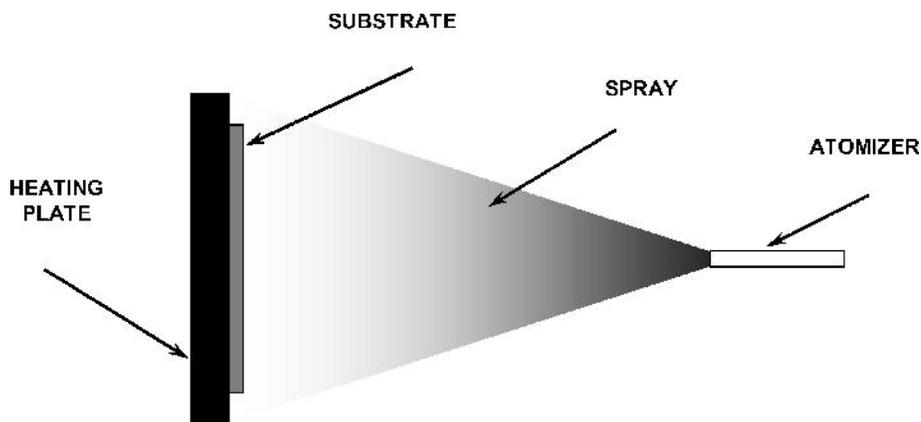
Fig 1: Schematic diagram of Chemical Spray Pyrolysis
