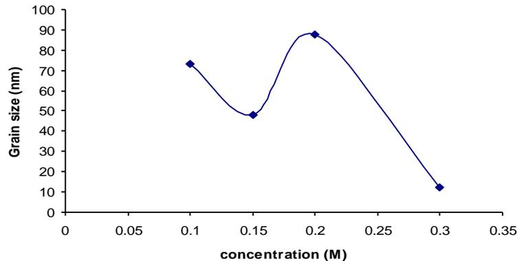
**Fig 5: Variation of grain size with concentration**
