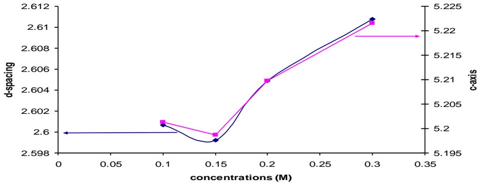
From the above graph, we can understand that, when concentration increases the observed d-spacing and c-axis also decreasing and then maximum point.
