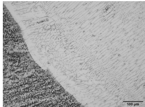
Fig-7 Microstructure of Interface stellite Metal - buffer SS309 - Buffer layer SS309 -200X
