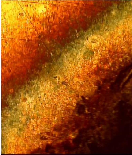
Figure 3. (100 x) H.A.Z. of a ASS 202-ASS
