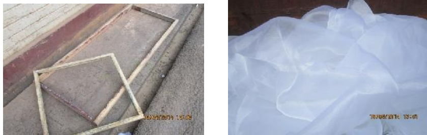
Figure 15: Wooden Screen Frame and White Screen Fabric/Mesh (Source: Fieldwork, 2021)
