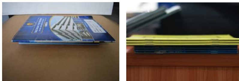
Figure 1: Saddle-wire Stitched Books showing the Staple Pins at the Edges (Source: Fieldwork, 2021)
