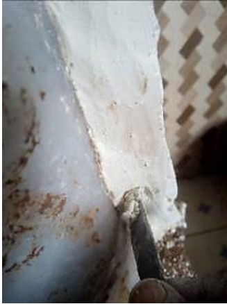
Fig 16. Creating a lock on the sim-line separation, on the Plaster of Paris, in readiness the second part of the plaster of Paris application for mother mold.
