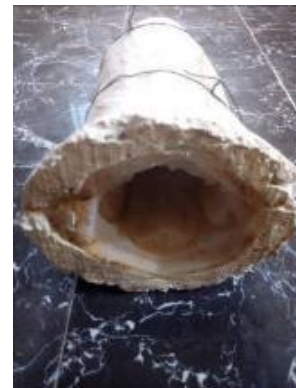
Fig 24. The silicon is properly positioned inside the mother mold, properly tied in preparation for casting.
