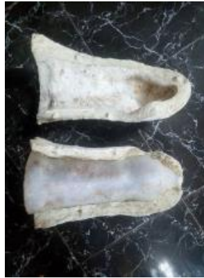
Fig 20. The Plaster of Paris, mother mold is separated and ready for the liberation of the trapped clay.
