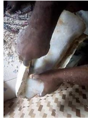
Fig 21. Silicon is cut at the sim-line with a sharp knife to enable it separated from the cast.
