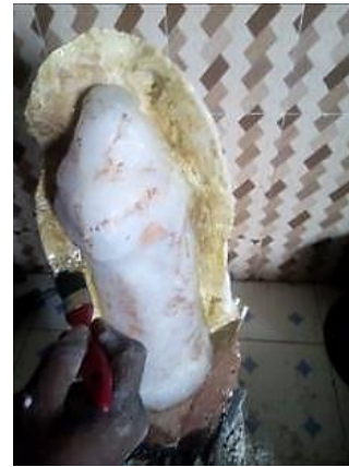
Fig 18. Applying lubricant on the Plaster of Paris for ease of separating the mother mold.
