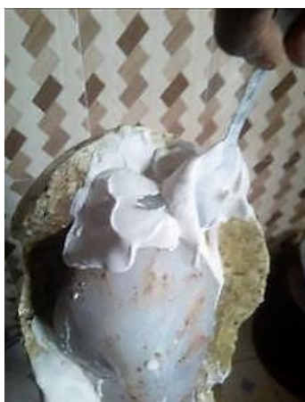
Fig14. Plaster of Paris is applied on the second part of the mother mold, with the aid of the spoon
