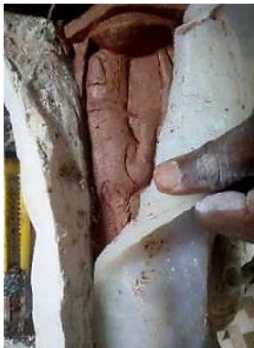
Fig 22. The clay is revealed inside the silicon, with the mother mold holding intact the flexible silicon.
