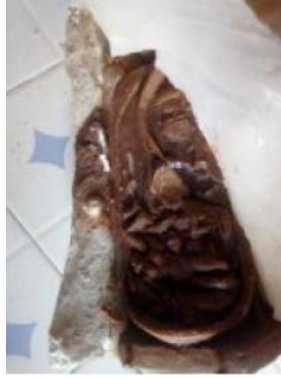
Fig 26. The polyester is revealed inside the silicon and ready to be liberated from it.
