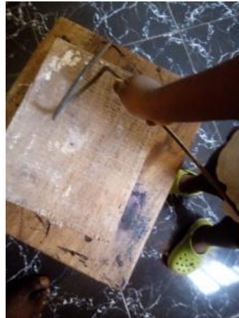
Fig 2. Construction of amature with flexible mild steel rod.
