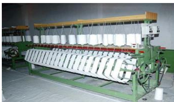
Figure 2. Electrical and Hand driven Hank reeling machines
