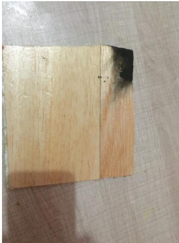
Fig. 1.4 Specimen after Fire Retardant Test
