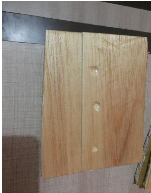
Fig. 1.3 Specimen after Hardness Testing using Rockwell Hardness Tester
