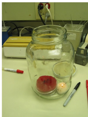
Candle jar: A candle is lit in a jar with a culture plate. The lid is put on, as the candle burns it increases the carbon dioxide levels in the jar.
